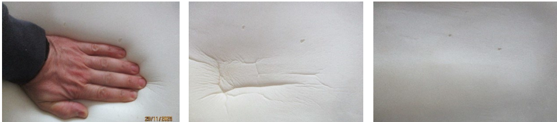
Figure 4. Memory property of a viscoelastic foam. The hand is involved by the foam, and after removing the hand, the foam returns to its original shape. Photos: Paulo Ramos.
